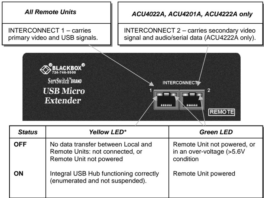
**Figure 3 Remote Unit - front view**
