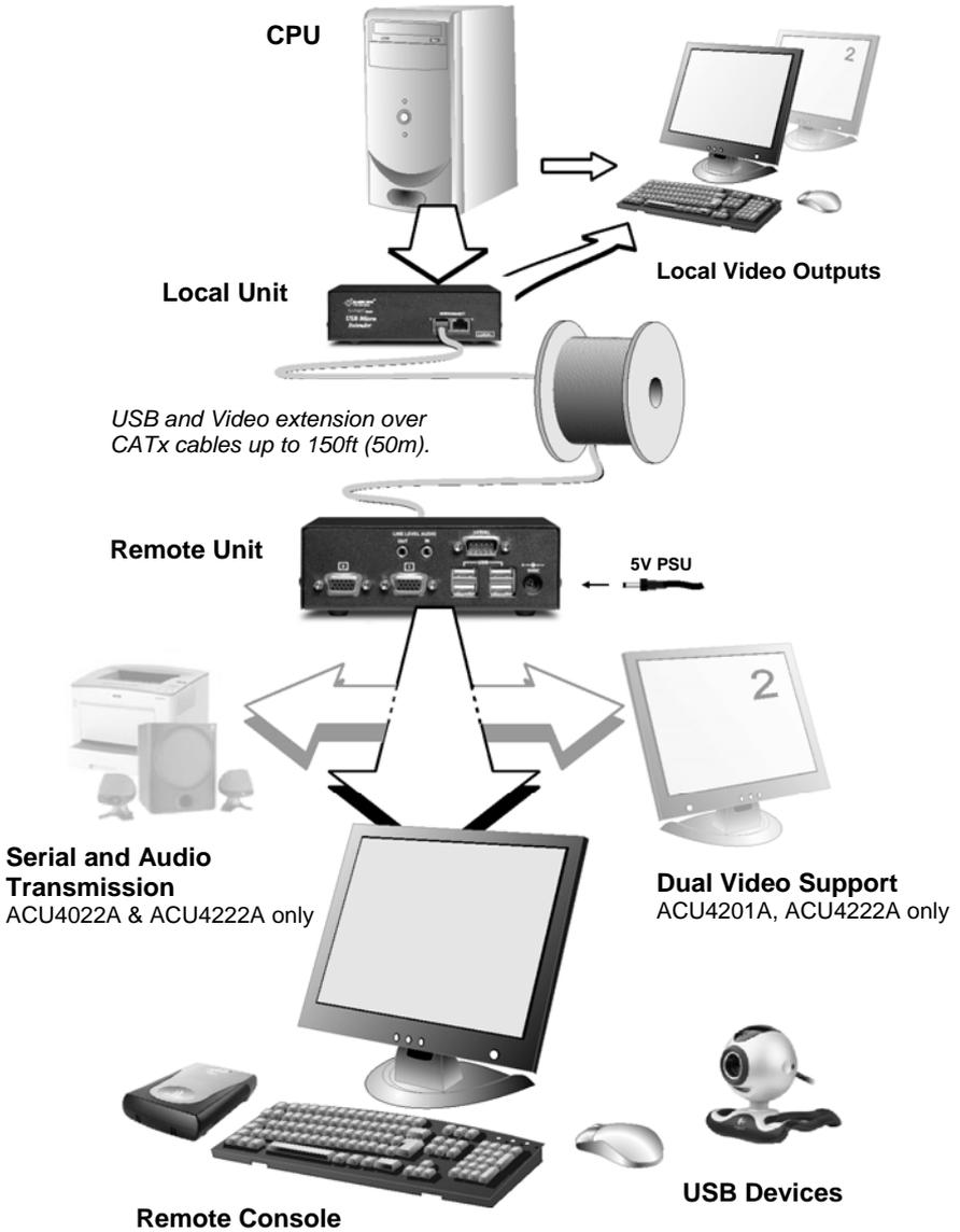
Figure 1 USB Micro Extender System
