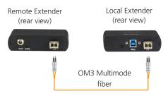
Figure QS-7. Connect local and remote extenders.
