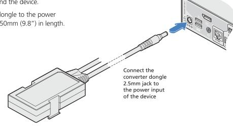
ACR1000-12V5-CBL2M or ACR1000-12V5-CBL5M - the latter has a longer (5m) cable) converter dongle
