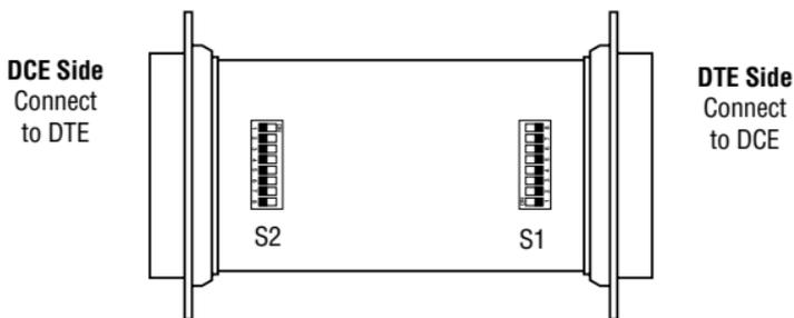
The two sets of DIP switches will be referred to as S1 and S2. The illustration below shows the orientation of DIP-Switches S1 and S2 with respect to ON and OFF positions.
